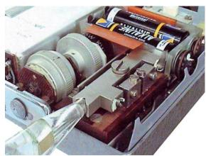
Detail view of the lever and paddle mechanism. During transport the paddle could be removed.
